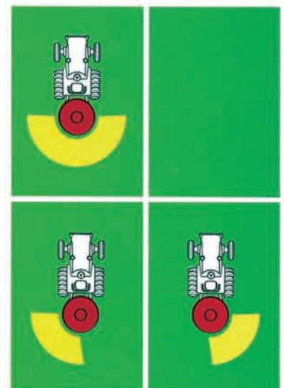
Average output per hour: 3/6 Ha. Fertilizer spreading quantity: adjustable from 20 up to 3700 Kg/Ha. Working speed: 3/16 Km/h with P.T.O. at 540 RPM.
